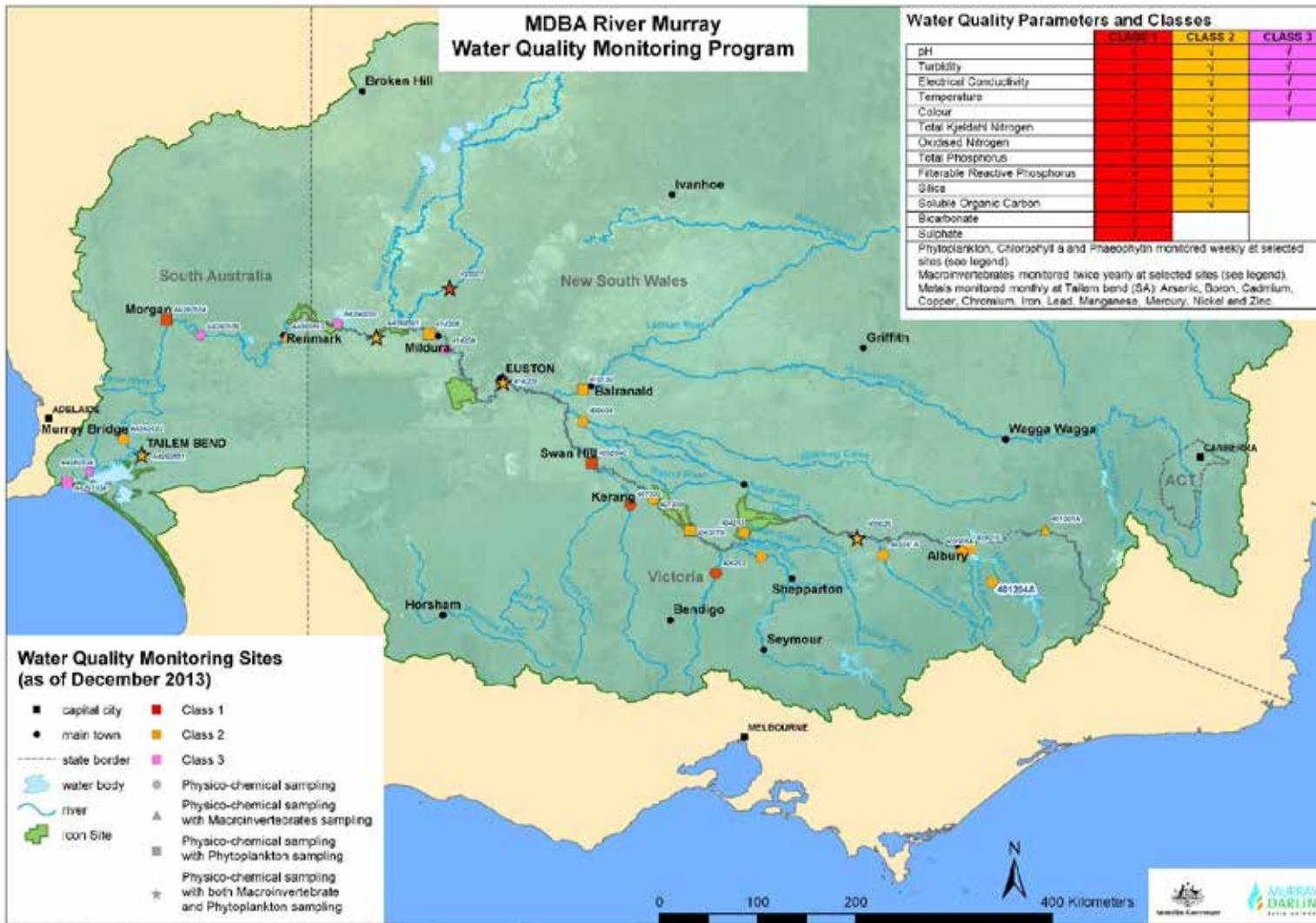
Figure 2: Revised Water Quality Monitoring Program sites, parameters and frequencies
