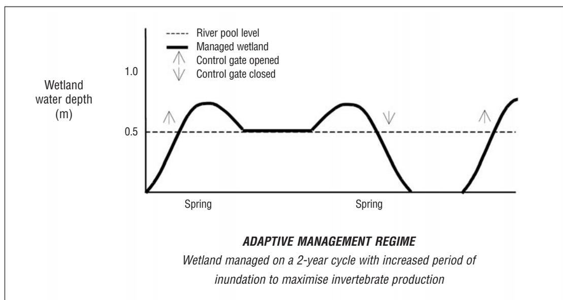
Figure 5. Wetting and drying cycle for Little Duck Lagoon provides a maximum of 14 months wet and 6 months dry over a 2 year period, timed to coincide with natural cycles in the main-stream. (Source: Jensen 2002b).
