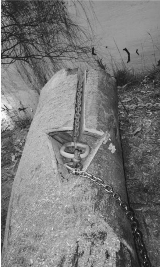
Figure 2. Quick release mechanism and cut used for easily retrieving the cable when the SWH item is in the correct position
