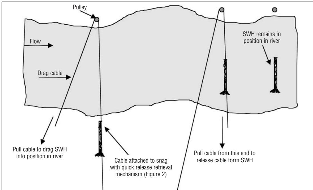
Figure 3. Cable dragging technique for placing snags
