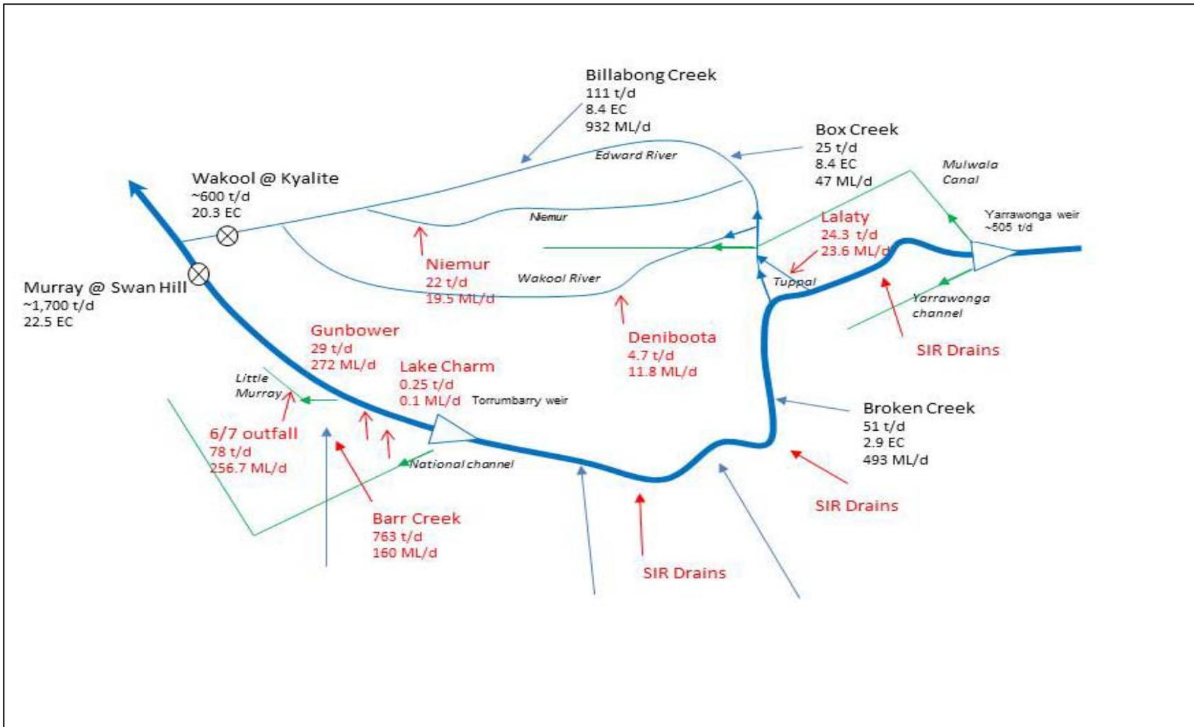
Figure 3: Schematic of BigMod drain inflow sources over benchmark period
