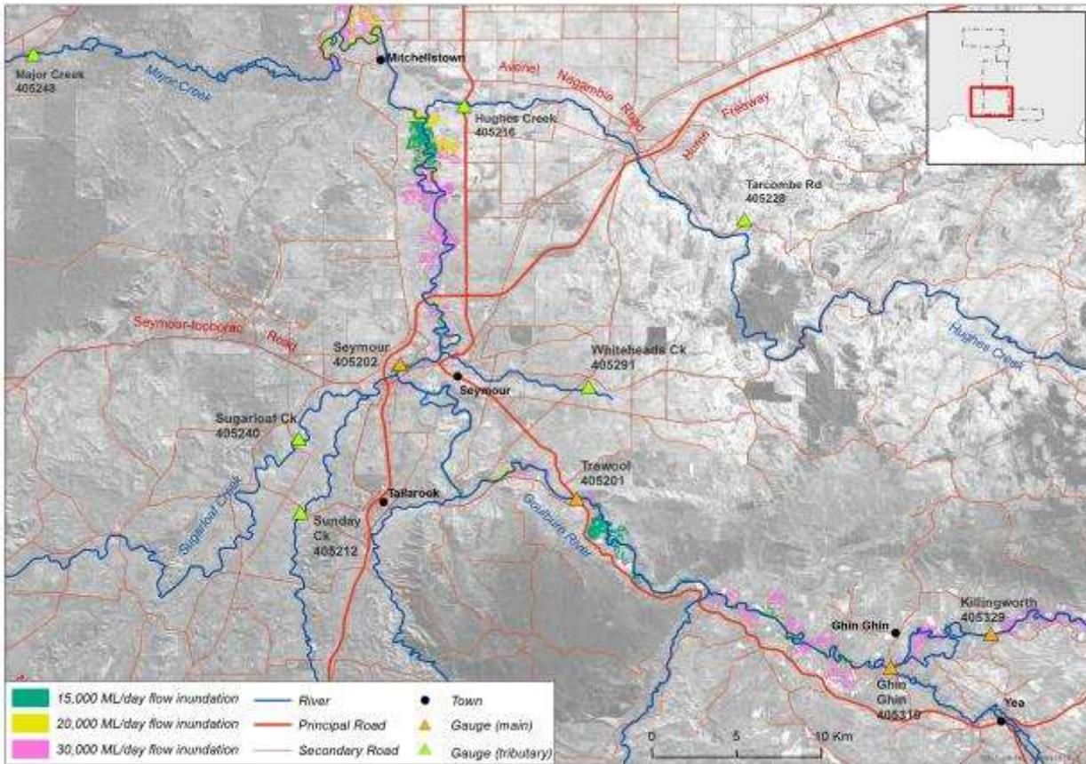
**Figure 28 a and b** Flow footprints for flows of 15,000, 20,000 and 30,000 megalitres (ML)/day between Killingsworth and Mitchellstown
