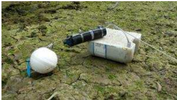
Figure 3: Typical deployment of VR2W receiver in a creek bed prior to inundation showing the concrete anchor and float.
